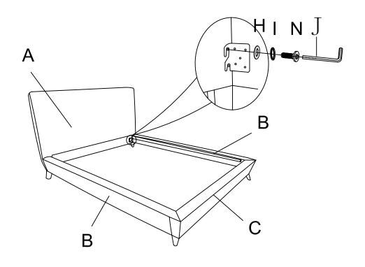
**STEP 5:** Attach Center slat rail (F) to Headboard (A)Footboard(C),using Allen bolt (N)with Flat washer (H),then fasten by Allen key(J)
