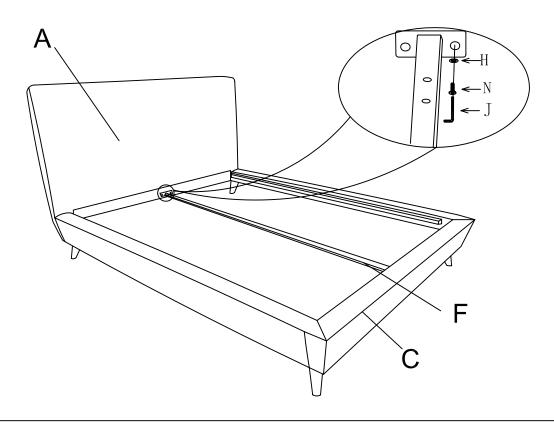
Attach Support leg (E)to Center slat rail(F),using Allen bolt (N)with Flat washer(H)and Nut (L),then fasten by Wrench
