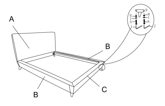
Attach Rail (B)to Headboard(A)and Footboard(C),using Allen bolt (N)with Flat washer(H)and spring washer(I),then fasten by Allen key(J)
