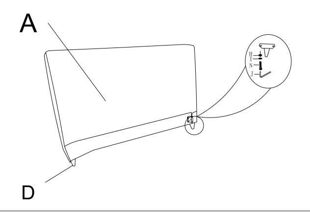
**STEP 2:** Attach leg(D) to Footboard(C),using bolt(N) with flat washer(H) and spring washer(I),then fasten by allen key(J).
